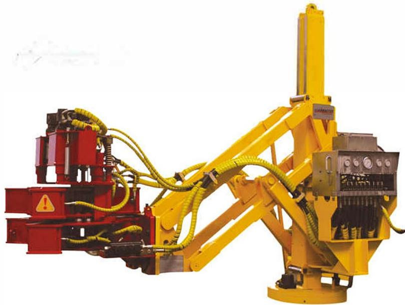
LM-120 Iron Roughneck is widely used during land and marine petroleum drilling operation, LM-120 Iron Roughneck is a wellhead instrument for operating makeup and breakout on drilling string (drill pipe, collar, casing and various tool joints) with caliber size of 3 1/2" ~9 5/8" . It can greatly reduce labor intensity of workers while operating trip out and trip in on drilling platform, and also improve the operation safety and efficiency.
